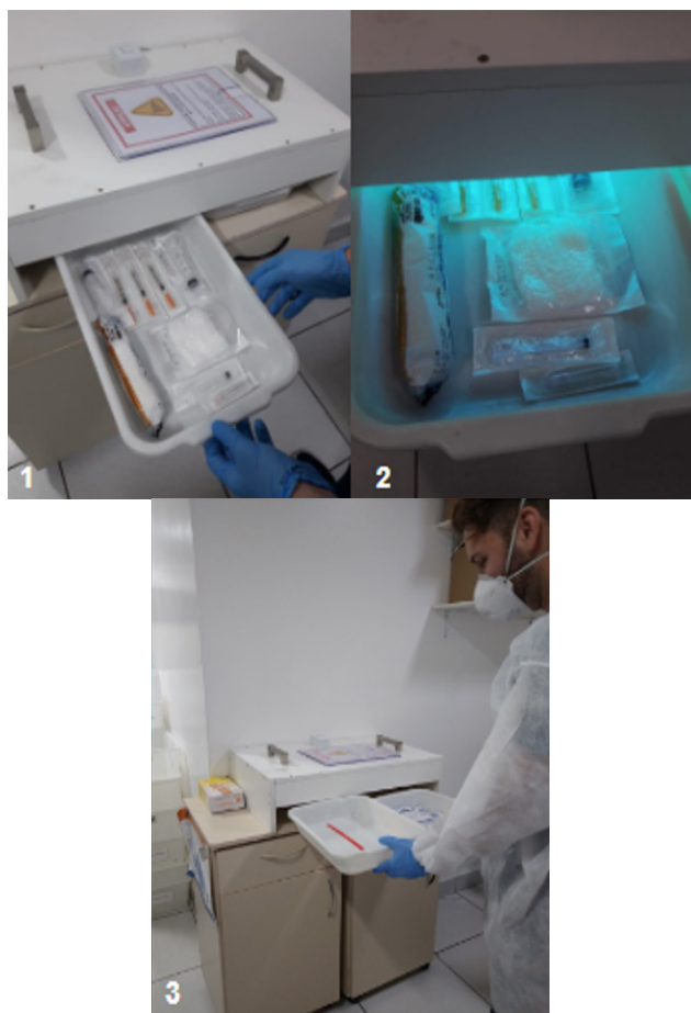
Figure 1. "UVC box" for disinfection of supplies returned to the pharmacy: portable device at different angles (1, 2 and 3) with two 18W lamps each.
