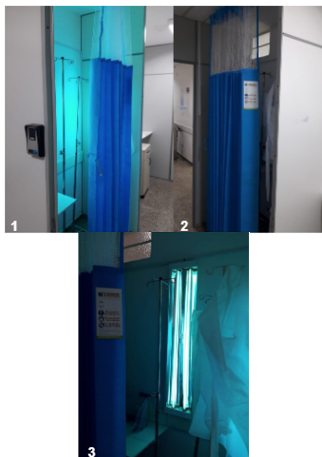
Figure 2. "UVC closet" with motion detector device at different angles (1, 2 and 3), for disinfection of gowns in the COVID-19 area: two UVC lamps of 60W each.
