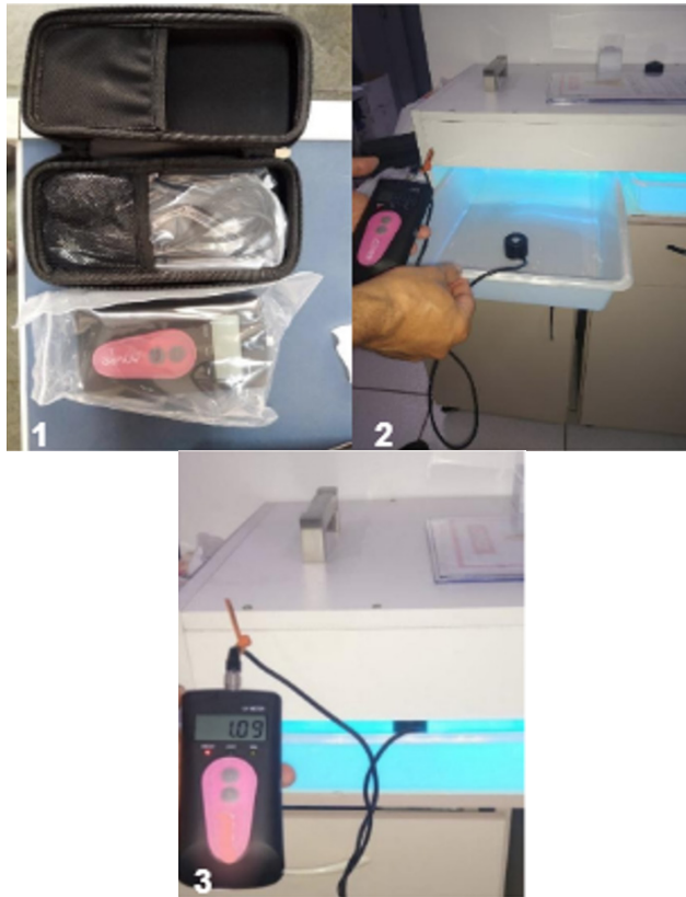
Figure 3. Different angles (1, 2 and 3) of the radiometer used to measure the power and radiation dose of the "UVC box": essential for full control of the use of lamps.
